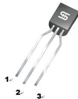
1. Collector 2. Base 3. Emitter TO-92 Plastic Package
